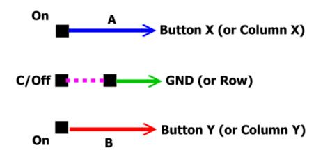
Looking at the above diagram of a 3 position (centre off) switch, it's possible to replicate the position 4, 5 & 6 switch states in the truth table. **Switch Down**, B is in contact with the common (position 4) **Switch Off**, neither line is in contact with the common (position 5)
