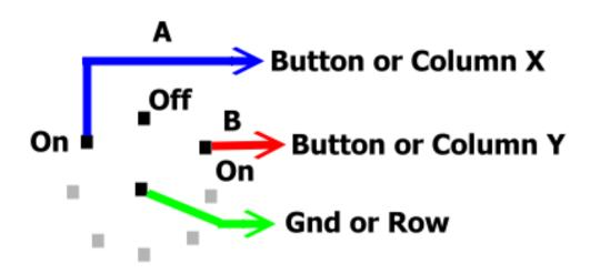
Result is a directional 3 way switch which inputs to Button X at each movement one way and Button Y at each movement the other way. So it's off to FSUIPC and record the macro's :o))
