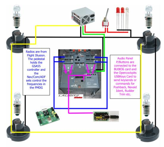
The Pedestal contains an ATX 650w PSU. This is switched on and off by a Toggle on the F/O Audio Panel. This gives me 12v for backlighting using MES Bulbs, 5 and 3v for LED's and also feeds the Flight Illusion GSA55 Interface Board
