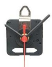
Place the washer onto the hub and gently tighten the nut so that the clock movement is firmly in place in the face plate.
